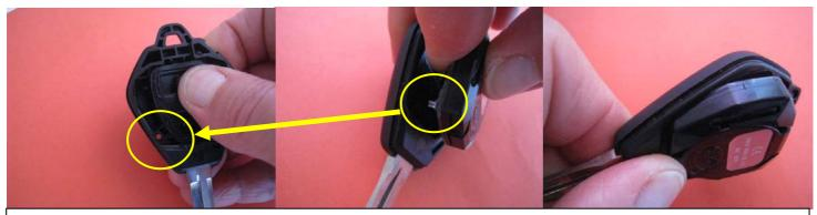
Place electronic component on the top of the Silicone Pad taking care of the little light that should gently fit in the hole provided (*as highlighted above*).
