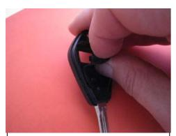
Continue the same process for second cut-out till last section of the new replacement pad engages with plastic cover.
