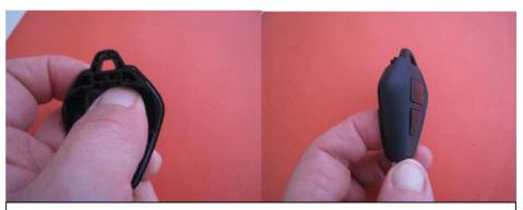
Push buttons slightly thru cut-outs till they look levelled with surface of the shell. Once Buttons pad is installed and buttons sit correctly, you can put your remote key together in reverse order.
