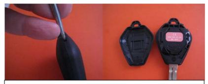
Use flat screwdriver to prise remote open on the split line. You will end up with bottom part of shell and top shell with buttons and electronic board.
