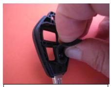
Start installing new pad by pushing one end of it under cut-out in plastic shell, till it stays in place
