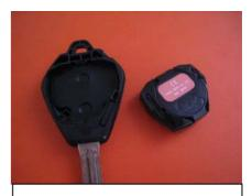
Remove electronic component from top shell and uncover thin rubber spacer.
