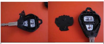
Remove rubber spacer and existing worn buttons. With our flexible Silicone Pad, rubber spacer will not be need it.
